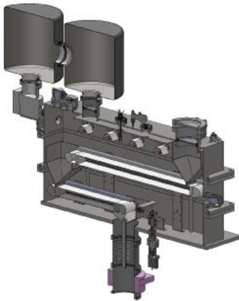
The dust preparation module
