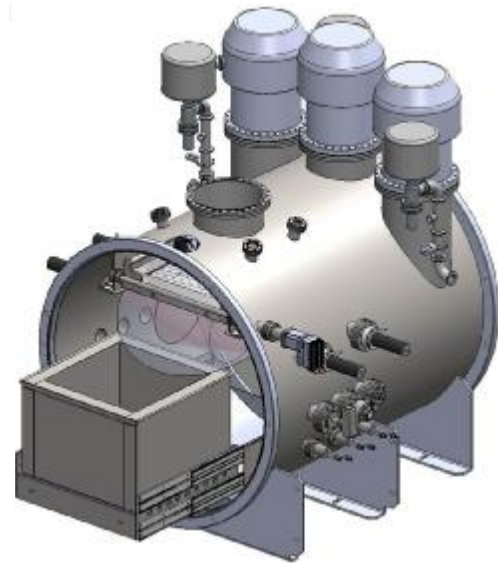
The Vacuum Chamber with the Test Rig/Sample Holder Box
