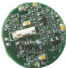
— internal design showing the microgravity sensor
