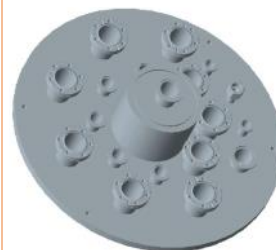
Fig. 8: T-Vac Chamber base plate
