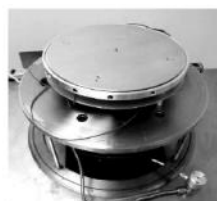
Fig. 6: Conceptual Configuration of Lunar Dust Simulator Facility (left) and Thermal control platform with TVAC dust tester (right)
